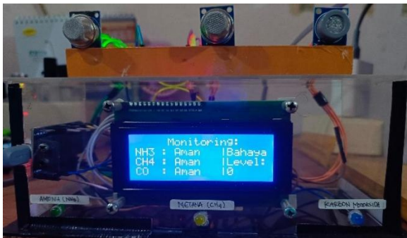
Fig.7. Gas Status Monitoring Results Using Fuzzy Sugeno Logic on the LCD
